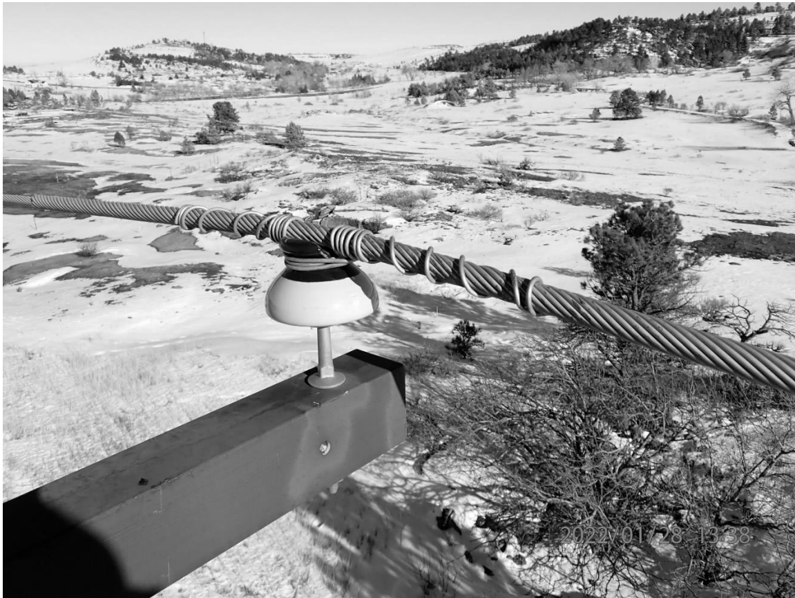
Figure 20. East phase conductor. Note that the lashing on this conductor had degraded and failed at the time of the fire and allowed the conductor to become displaced from the insulator. The lashing on the conductor was replaced after the fire.
