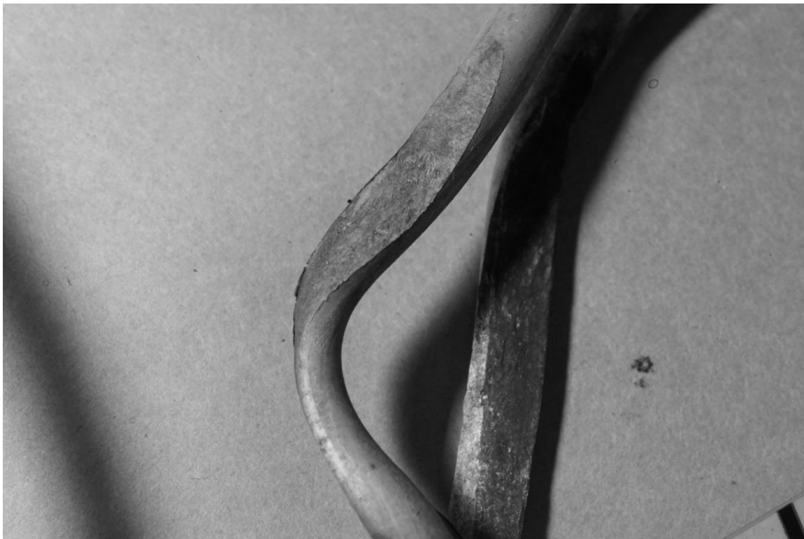
Figure 22. Failed lashing from the east conductor with evidence of wear and electrical arcing.
