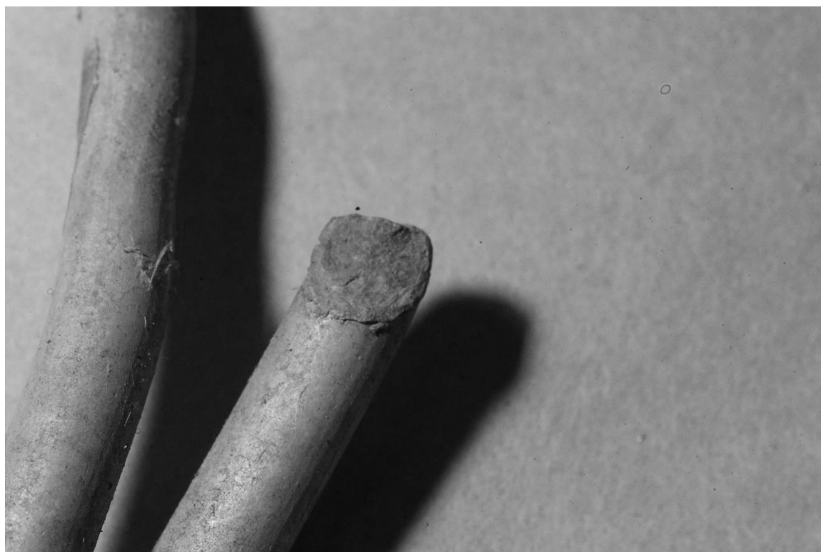
Figure 23. Evidence of electrical on the failed lashing.
