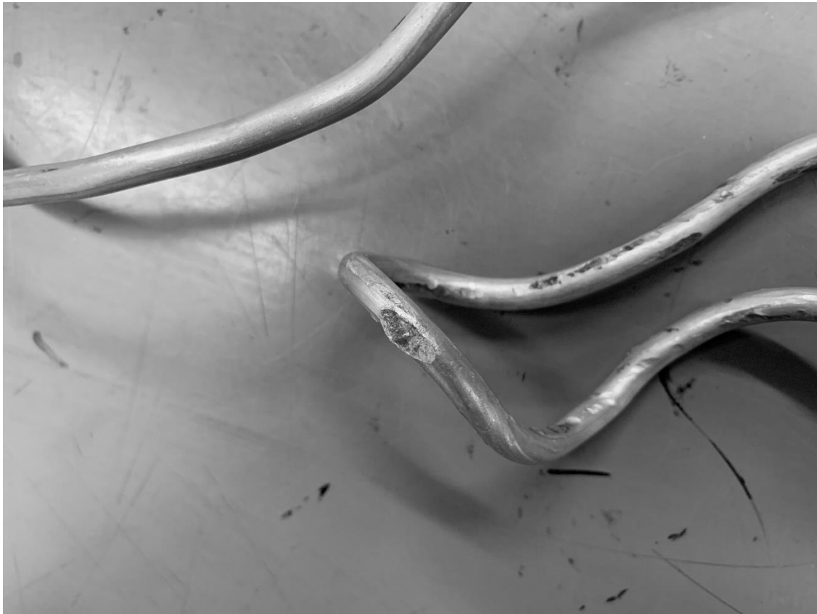
Figure 24. Evidence of electrical on the failed lashing
